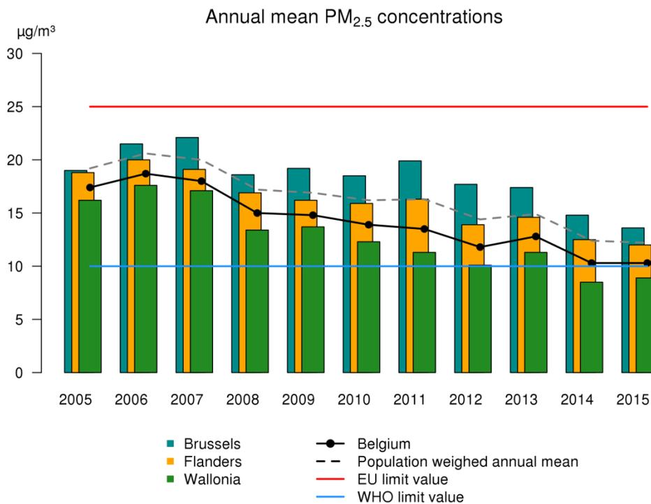
**Figure 21: Evolution of the spatially averaged annually mean PM<sub>2.5</sub> concentrations for the three Regions and Belgium, and of the population-weighted annual mean concentration for Belgium. All data were calculated using the RIO interpolation technique.**
